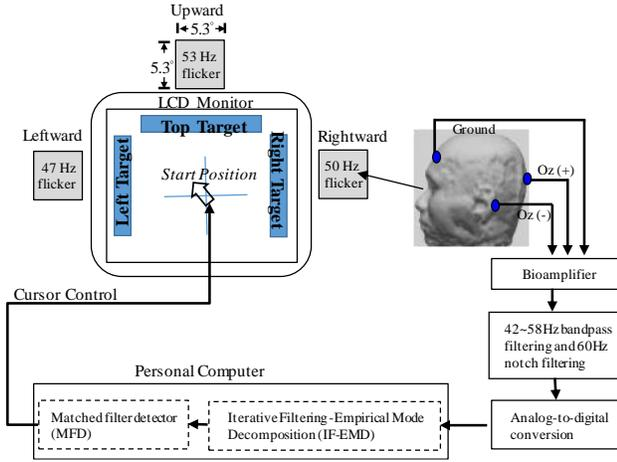
Figure 1. Architecture of the proposed IF-EMD SSVEP-based BCI system..
