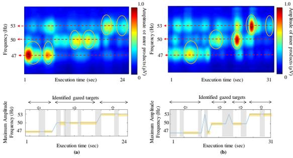
Figure 2. The  $b_m$  and detected  $b_{max}$  of application task in subject II and subject III are shown in Fig. 2a and Fig. 2b, respectively. Upper panel: the time course of bm; Lower panel: the recognized targets of valid commands.
